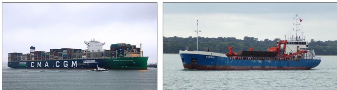
Figure 34: Left - CMA CGM Jacques Saade– 400m LOA x 61m Beam, right - Al Avocet (called Karissa until recently) – 100 m LOA x 12m.
